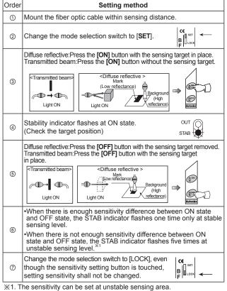
※ When the power is OFF, the set sensitivity is saved.
