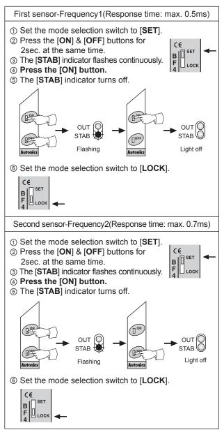
• Interference prevention function (Operation of normal mode)
