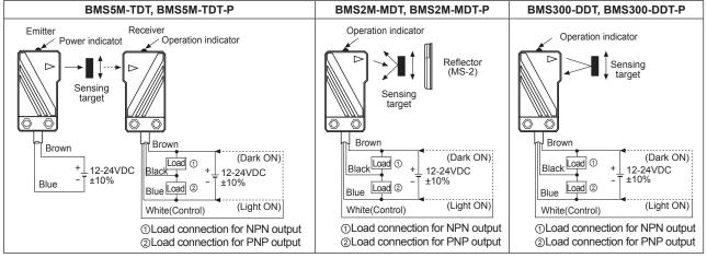
% Dark ON mode is on when control line is opened.
