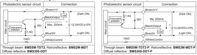
% Select Light ON / Dark ON by control wire. - Light ON : Connect control wire to 0V / Dark ON : Connect control wire to +V
