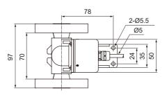
Cable for axial cable type Ø5mm, 4-wire, Length: 2m, Shield cable Cable for axial cable connector type
