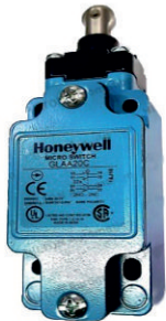
GLAA20C TOP ROLLER PLUNGER 2NO + 2NC
