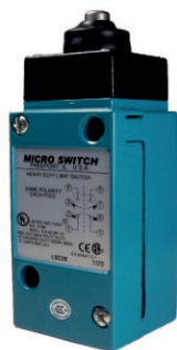
LSC2B TOP PIN PLUNGER MOMENTARY (0.75 - 14 NPT) 2NO 2NC
