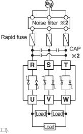
%2: When connecting noise filter and capacitor, it is appropriate for EMC.
