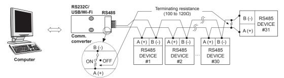
%It is recommended to use Autonics communication converter; SCM-WF48 (Wi-Fi to RS485. USB wireless communication) converter, sold separately), SCM-US48I (USB to RS485 converter, sold separately), SCM-38I (RS232C to RS485 converter, sold separately). Please use twisted pair wire, which is suitable for RS485 communication, for SCM-WF48, SCM-US48I and SCM-38I.
